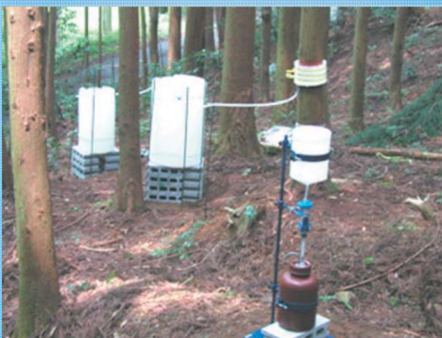
A throughfall/stemflow collectors (left) and stream water sampling point (right) at the Ijira Lake catchment
