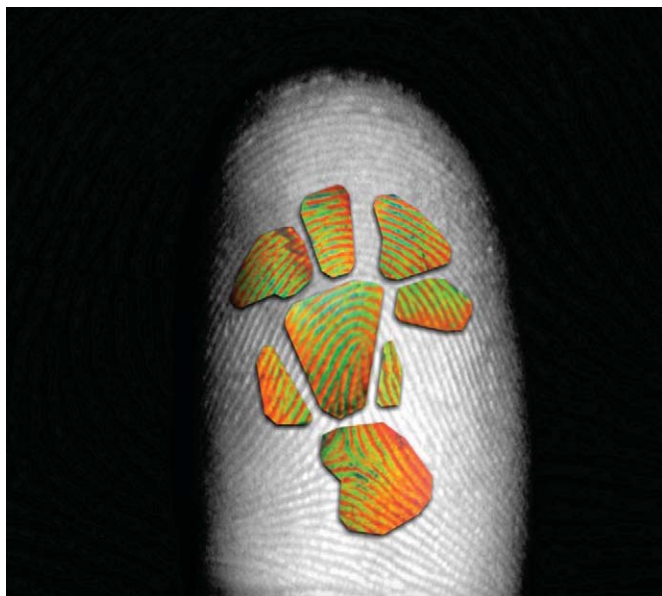
Fig. 9 A full-color fingerprint visualized using an elastic photonic crystal, overlaid onto a grayscale image of an index finger.
