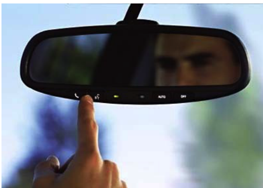
The 2004 Chrysler Pacifica features an auto dim electrochromic rearview mirror. PHOTO COURTESY DAIMLERCHRYSLER
