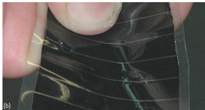
Fig. 2 Examples of flexible (a) CIGS test cells (b) and an integrated module (courtesy of ZSW 24 ). Under full-sun illumination, cells on the PI foil reach \eta = 11\% 21 and those on stainless steel achieve \eta = 17.4\% 18 . Monolithic series connection of the cells yields a module efficiency of \eta = 6.8\% 21 .
